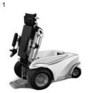
The product allows for fast and easy adjustment of seat depth and lower leg length. It enables the operator to achieve an upright posture, with unrestricted shoulder movement when swinging a golf club.
